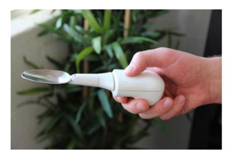
This device, developed by Lift Labs, contains microelectronics in the base that allow it to cancel out the effects of hand tremors suffered by essential tremor patients. Credit: Lift Labs
