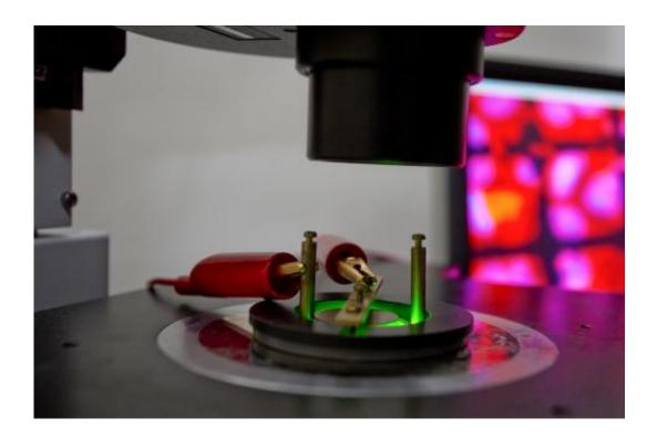
This is a micro-fabricated device for live imaging of single cell response during electrical stimulation. Credit: Dottie Stover, U. of Cincinnati
