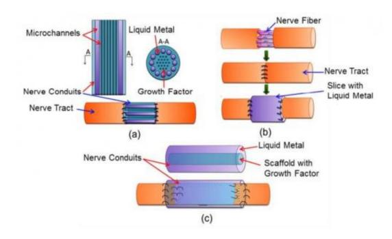
Three kinds of nerve conduits to repair the injured peripheral nerve. (a) Nerve conduit with microchannels. (b) Nerve conduit with a shape of thin slice. (c) Nerve conduit with concentric tubes. Credit: arXiv:1404.5931 [physics.med-ph]
