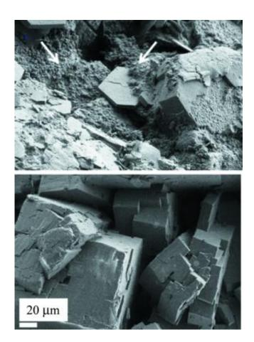
This is a SEM image of stones treated by 2 different drugs. Above you see altered crystals with a rough surface, below, you see crystal edges still well defined, suggesting limited effect of treatment. Credit: Dominique Bazin et al
