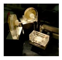
Prototype droplet network printer built by Oxford scientists. Credit: OU/G Villar
