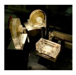
Prototype droplet network printer built by Oxford scientists. Credit: OU/G Villar
