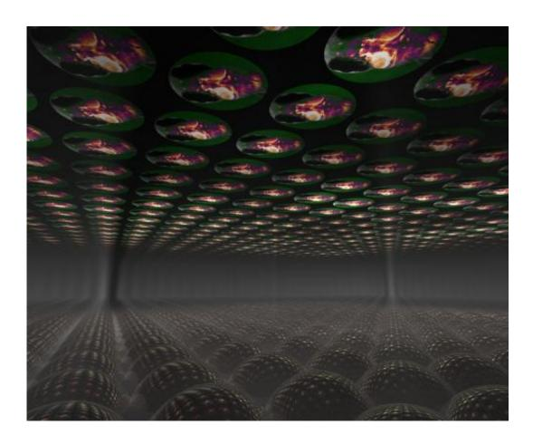
A microlens array captures different perspectives of the sample, in this case a live larval zebrafish
