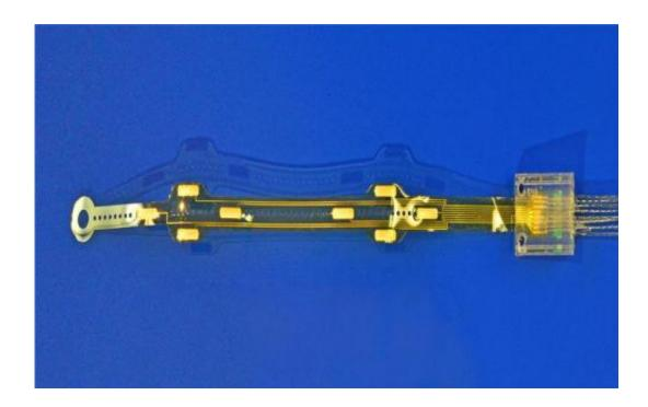
The implantable microelectrode sensors are flexible and wafer-thin. Credit: Fraunhofer IMM
