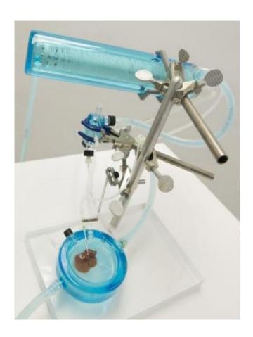
The liver is perfused with a solution in this pump system before and after supercooling preservation. The blue color is caused by antifreeze that surrounds the components of the system to regulate the temperature. Credit: Wally Reeves, Korkut Uygun, Maish Yarmush, Harvard University
