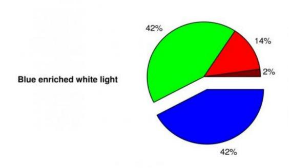
On the left, the spectrum of the white light consists of roughly equal parts of red and green (about 40 percent), then blue (12 percent) and infrared waves (4 percent). On the right, the proportions are different (42 percent blue and 14 percent red). Nevertheless, with the naked eye, a human will perceive a white
