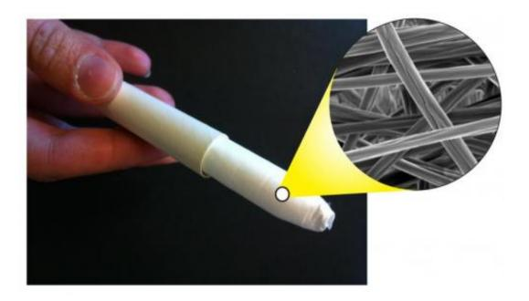
The UW's dissolving fibers could be spun and placed within an applicator, similar to those used to insert a tampon. The inset image shows the quick-release fibers magnified 5,000 times. Credit: U of Washington
