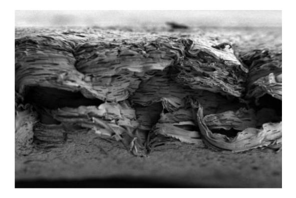
Pictured is a scanning electron micrograph of a porous, nanostructured poly(lactic-co-glycolic acid) (PLGA) membrane. The membrane is coated with a polyelectrolyte (PEM) multilayer coating that releases growth factors to promote bone repair. Credit: Nasim Hyder and Nisarg J. Shah
