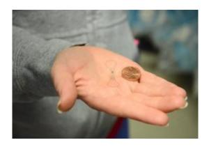
The CardioMEMS device is shown next to a penny for scale.
