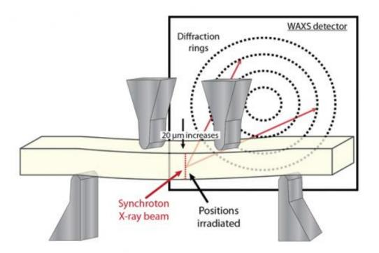
Schematic of mechanical testing apparatus utilized during collection of WAXS diffraction data at the APS. Bone beams were subjected to 4-point bending, and after each displacement of 20 mm (black arrow), 20 x-ray scattering measurements were taken (red dashed line). Diffraction patterns collected by the detector (indicated) allow for quantification of strain experienced by hydroxyapatite crystals and mineralized collagen within the bone. Adapted from M.A. Gallant, Bone 61, 191 (2014).
