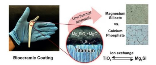
The artwork appeared on the front cover of Applied Surface Science summarizes the benefits of a new bioceramic coating versus the commercially available Calcium Phosphate which develops microcracks during processing and may later cause osteolysis in load-bearing orthopedic implants.
