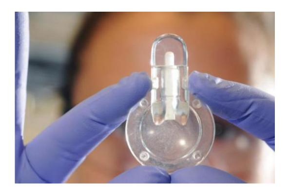
This is a close-up of a prototype device for point-of-care testing of anemia. The device could enable more rapid diagnosis of the common blood disorder and allow inexpensive at-home self-monitoring of persons with chronic forms of the disease. Credit: Gary Meek
