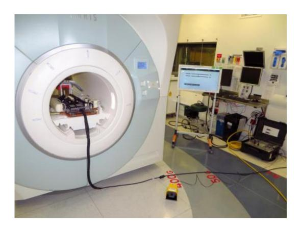
This is an overview of the MRI-compatible prostate biopsy robotic system developed by researchers at Worcester Polytechnic Institute (WPI), Johns Hopkins University, and Brigham and Women's Hospital. From left, the robot in place inside the MRI unit; the foot pedal the physician used to activate the robot; a screen that display's the robot's status, and (black case on floor) the robot control unit. Credit: Worcester Polytechnic Institute
