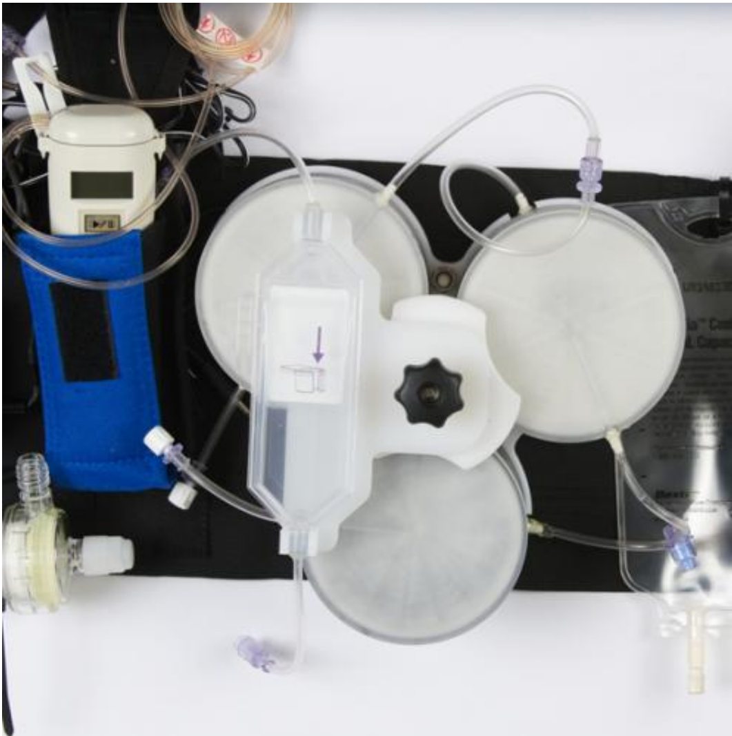
This detail shot shows the WAK's filtration system, right, and one of the auxiliary pumps, left. Credit: Stephen Brashear
