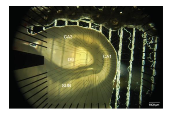
The 10 x 6 multi-electrode array developed by the USC Viterbi research team for experiments in recording epileptic seizures in human brain slices. Credit: USC Viterbi School of Engineering
