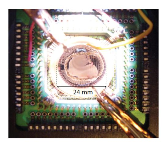
An epileptic human hippocampal slice submerged in the multi-electrode array recording chamber developed by the USC Viterbi research team for experiments in recording epileptic seizures. Credit: USC Viterbi School of Engineering
