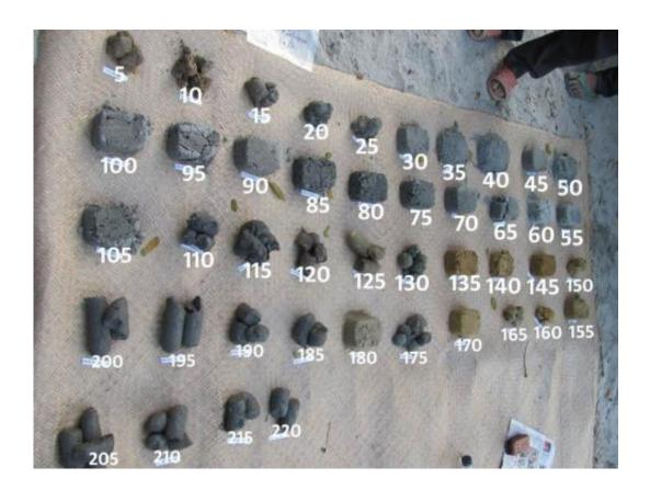
Sediment samples characterization for development of Sediment Color Tool and also targeting the sediments for installation of arsenic-safe tubewells. Credit: KTH Royal Institute of Technology
