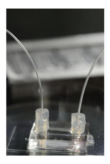
Tiny tubes connected to the chip carry a fluid that behaves like the bloodstream, allowing the Johns Hopkins researchers to study how metastasis occurs. Credit: Will Kirk/Johns Hopkins University
