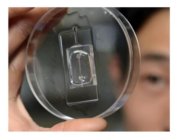
This dish houses a lab chip that Johns Hopkins engineers built to gain an unprecedented close-up view of how cancer cells enter the bloodstream to spread the disease. Credit: Will Kirk/Johns Hopkins University
