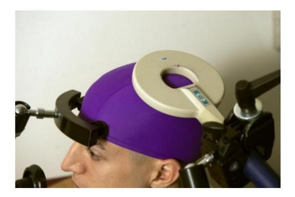
A transcranial magnetic stimulation coil is placed over the part of the brain that controls the receiver's right hand movements. Credit: U of Washington
