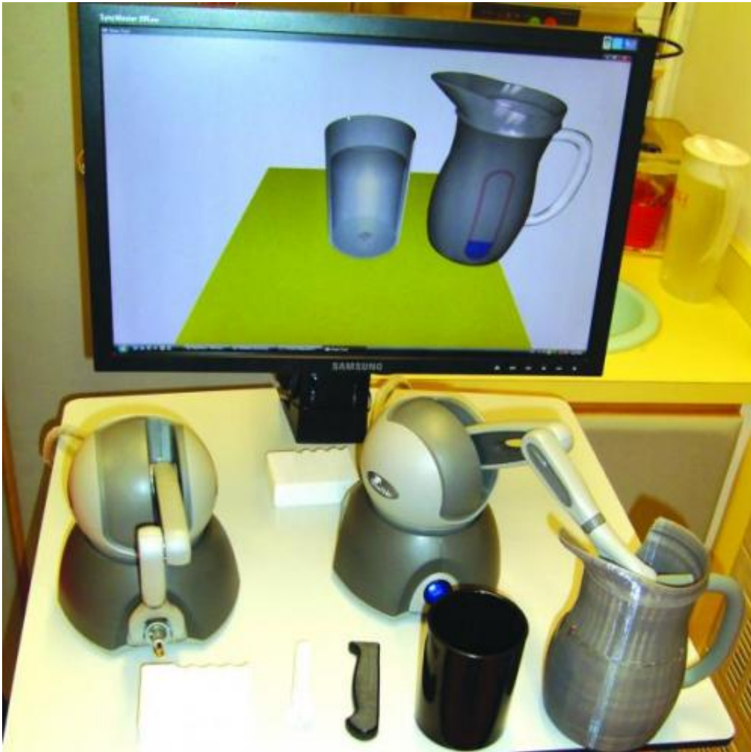
The prototype of the haptic platform customized for self-care training. Credit: The Hong Kong Polytechnic University
