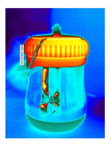
Thermal imaging of the NINA device was used to assess heat losses and compare insulating materials. Credit: Paul LaBarre, PATH
