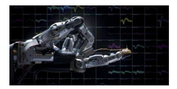
Researchers at the DPZ built this robothand. They analyse the brain activity of non human primates during the execution of hand grasping movements. This neuronal information, recorded with fine electrodes in the cortex, could one day be used to control a robotic hand as a prosthesis for paralyzed people. Credit: Sebastian Lehmann
