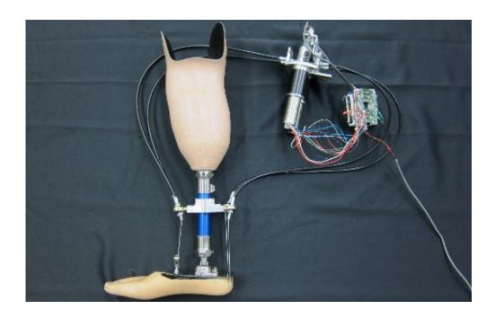
A portable computer-controlled actuator that can be carried in a pocket can help this robotic prosthetic ankle "see" where it is going.
