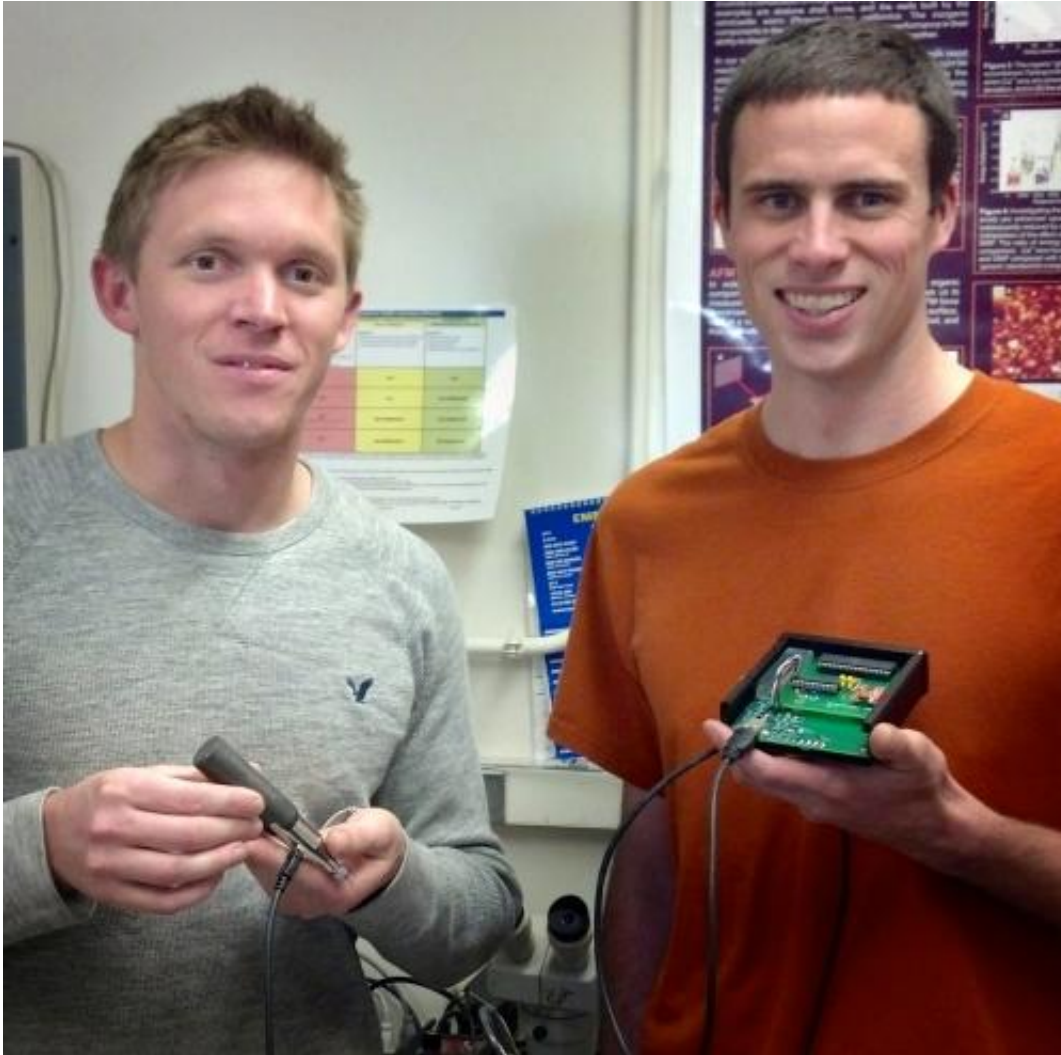
Co-inventors Connor Randall (left) and Daniel Bridges hold the instrument, which measures the bone material strength index. Credit: UCSB
