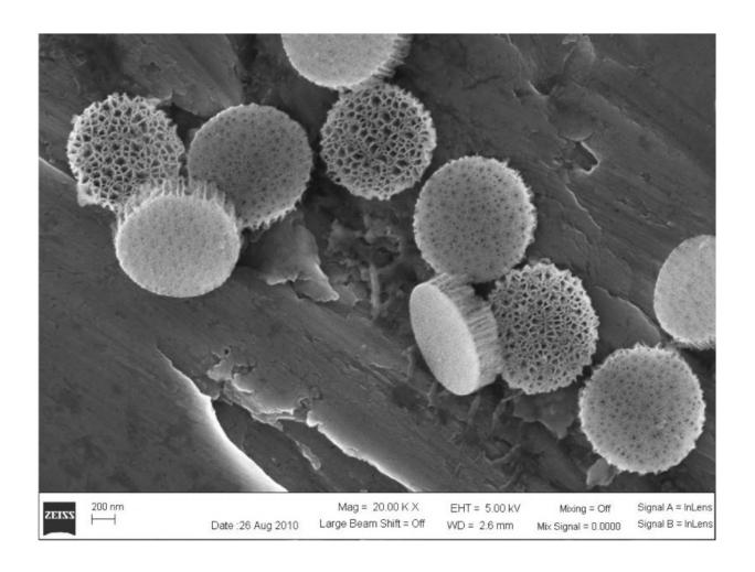
The porous silicon microparticles are about 1 micrometer in diameter. The hollow channels within each microparticle can be loaded with antigens -- such as HER2 -- that can help train the immune system to recognize and destroy cancer cells overexpressing HER2. Credit: Haifa Shen lab
