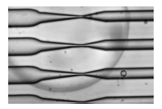
As cells pass through the CellSqueeze device at high speed, narrowing microfluidic channels apply a squeeze that opens small, temporary holes in the cells' membranes. As a result, large molecules — antigens, in the case of this study — can enter before the membrane reseals. Credit: SQZ Biotech
