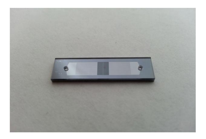
CellSqueeze's microfluidic channels are etched on silicon chips and sealed with a glass layer. The channels temporarily deform cells so molecules can enter. Credit: SQZ Biotech
