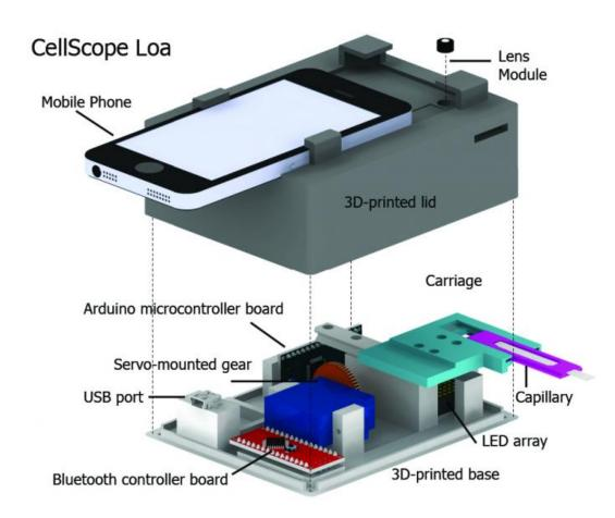
A schematic of the CellScope Loa device, a mobile phone-based video microscope. The device includes a 3-D-printed case housing simple optics, circuitry and controllers to help process the sample of blood. CellScope Loa can quantify levels of the Loa loa parasitic worm directly from whole blood in less than 3 minutes. Credit: Mike D'Ambrosio and Matt Bakalar, Fletcher Lab, UC Berkeley
