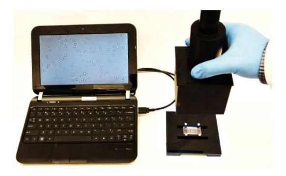
CD4+ T cells captured on the polyester film-based platform are imaged with the lensless device and are clearly visible on the attached portable laptop screen.
