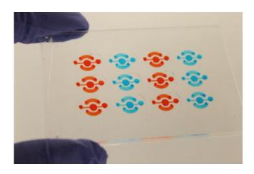
This microfluidic petri dish provides a highly accurate ex vivo testing environment.
