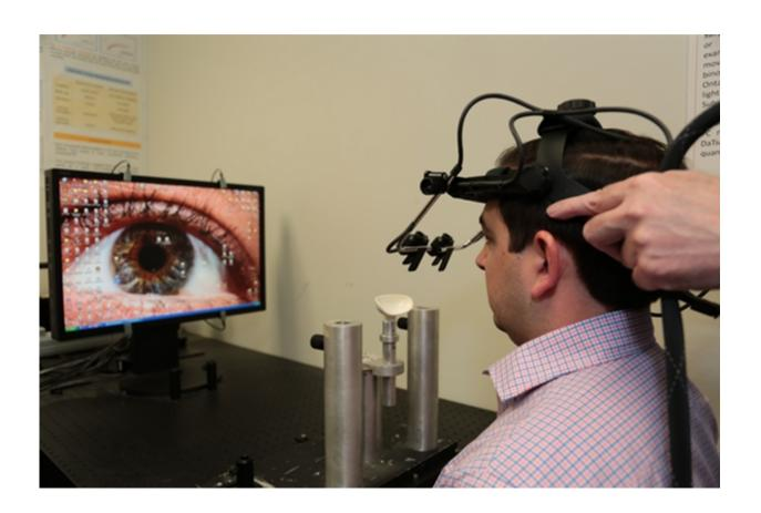
George Gitchel, a Ph.D. candidate in biomedical engineering at VCU, models an automated eye-tracking system that detects and analyzes eye movements as a means to accurately differentiate and diagnose more than 20 neurological diseases.
