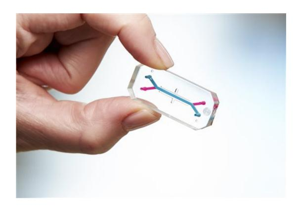
This undated product image provided by Johnson & Johnson shows Emulate's Organ-On-Chips technology, a computer chip designed to simulate functions of human organs to predict which experimental drugs are most likely to be effective and safe in people. The project is aimed at limiting the failure of drugs after they get into expensive testing in patients. (Johnson & Johnson via AP)
