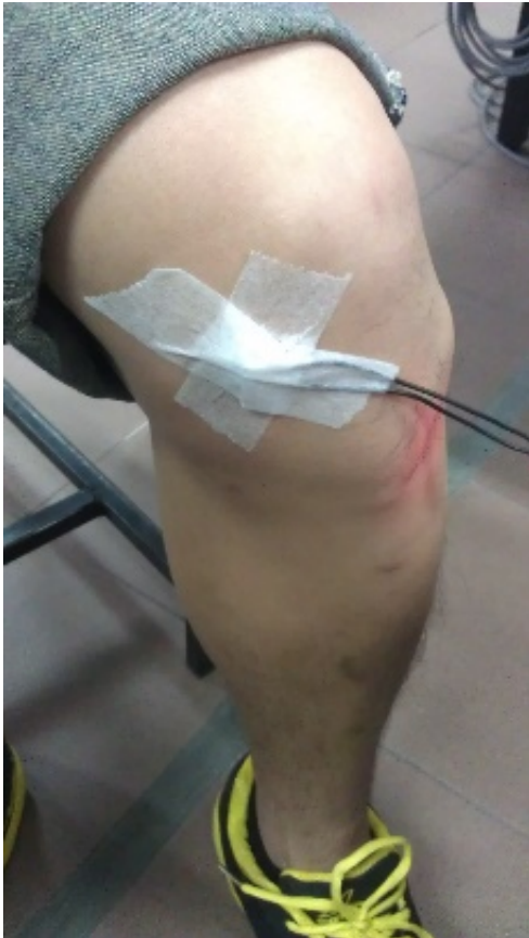
Microphone attached to subject's knee
