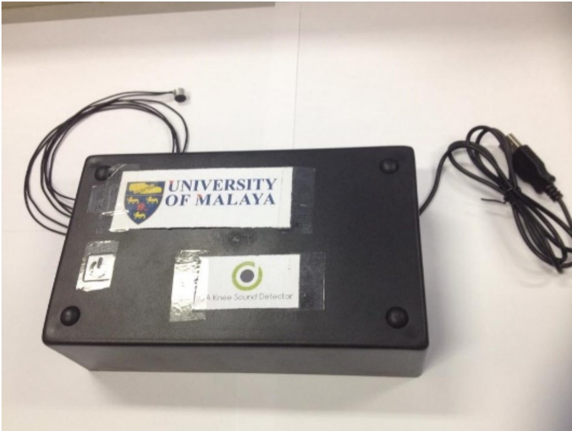
Knee Sound Detector device.
