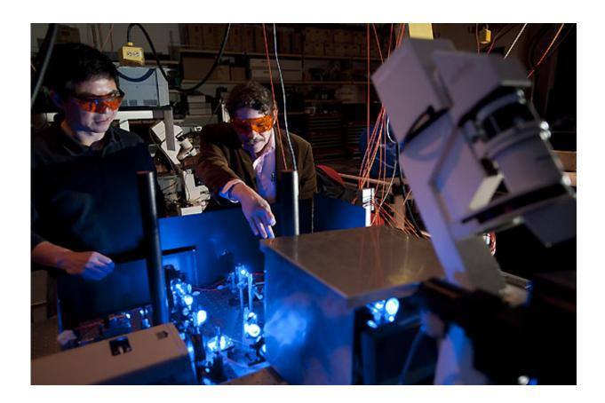
Shiguo Zhou (left) and David C. Schwartz look at the path that blue laser light follows -- through focusing optics and beam splitters -- before leading to one of their automated research microscopes in the Laboratory for Molecular and Computational Genomics at the University of Wisconsin-Madison. Credit: Jeff Miller/University of Wisconsin-Madison
