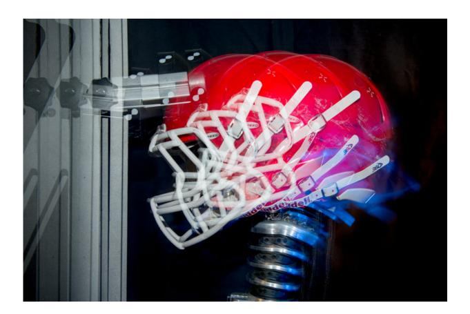
Stanford research suggests that current football helmet tests may miss concussionprone actions. The researchers are currently testing a new apparatus (above), consisting of a dummy head mounted on a biofidelic neck, that they hope will simulate more realistic field impacts. Credit: L.A. Cicero / Stanford News Service
