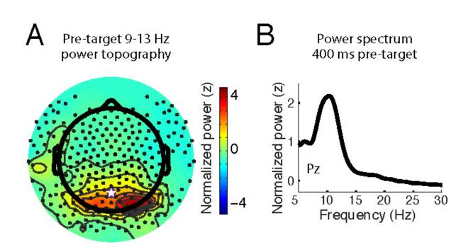
Fig. 3. Spatial and frequency specificity of the alpha-band signal. (A) Scalp topography of absolute alpha power 400 ms before target onset, with electrode Pz indicated. (B) FFT of the pretarget data, indicating a peak in power at 10.6 Hz. Credit: Samaha J et al. (2015) Top-down control of the phase of alpha-band oscillations as a mechanism for temporal prediction. *Proc Natl Acad Sci* USA 112(27):8439-8444.
