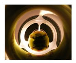
A ball is in the barrel of an air cannon before firing during testing in the lab.
