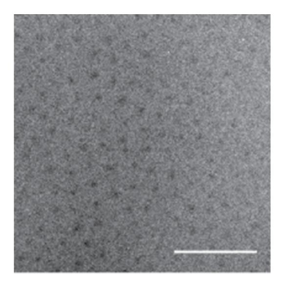
This is an image of the newly repackaged pharmaceutical under a transmission electron microscope. The dark spots are the water-insoluble cores of the nanoparticles, while the peptide chains are barely visible due to their low electron density and high degree of hydration. Credit: Ashutosh Chilkoti, Duke
