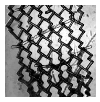
The honeycomb mesh of cells being compressed by contracting heart cells growing along the scaffold. Credit: Boyang Zhang/ University of Toronto Engineering
