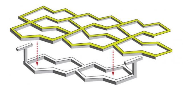
This diagram shows how the T-shaped posts on one layer of the tissue scaffold pass through the holes in a second layer. The mechanism is similar to the hooks and loops used to fasten Velcro<sup>TM</sup>. Credit: Raymond Cheah/ University of Toronto Engineering
