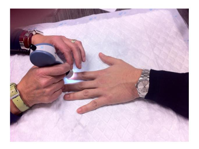
One prototype is a portable microscope which is placed manually on the patient's fingertip to take videos of microcirculation in very superficial capillaries. Credit: Research Laboratory of Electronics / MIT
