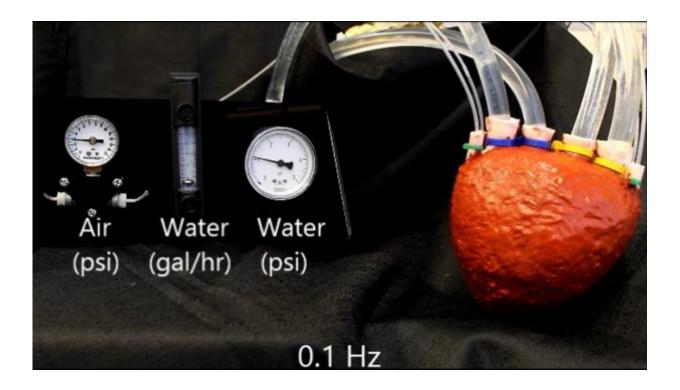
Artificial hearts with multiple moving parts increase the chance of failure; scientists have worked up a device which is a single piece. No less interesting is the material they used; the team is taking a page out of soft robots.
