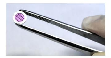
A silicon microsieve with densely packed pores can capture circulating tumor cells from blood. Credit: A\*STAR Institute of Bioengineering and Nanotechnology
