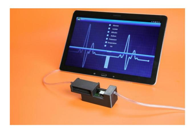
A device developed at EPFL that is capable of monitoring in real-time 5 vital substances for patients in ICU. Back: preview of the tablet app designed to monitor the values. Credit: Alain Herzog / EPFL 2015
