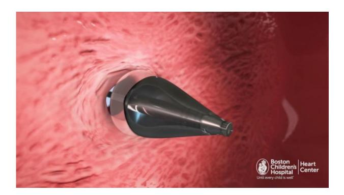
Harvard John A. Paulson School of Engineering and Applied Sciences (SEAS) and the Karp Lab at Brigham and Women's Hospital have jointly designed a specialized catheter for fixing holes in the heart using a biodegradable adhesive and patch. Two balloons, one on either side of the hole, open and apply pressure to the patch to secure it in place. Here, the right balloon is being deployed. Credit: Boston Children's Hospital
