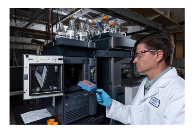
Georgia Tech research scientist David Gaul places samples into an ultraperformance liquid chromatography-mass spectrometry (UPLC-MS) instrument for testing. The UPLC-MS technique was used to help identify 16 metabolites associated with early-stage ovarian cancer. The work, utilizing serum samples, could lead to an accurate screening test for the disease. Credit: Rob Felt, Georgia Tech
