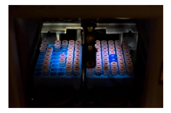
Samples are shown ready for testing in an ultra-performance liquid chromatography-mass spectrometry (UPLC-MS) instrument in the laboratory of Facundo Fernández at the Georgia Institute of Technology. The UPLC-MS technique was used to help identify 16 metabolites associated with early-stage ovarian cancer. The work, utilizing serum samples, could lead to an accurate screening test for the disease. Credit: Rob Felt, Georgia Tech
