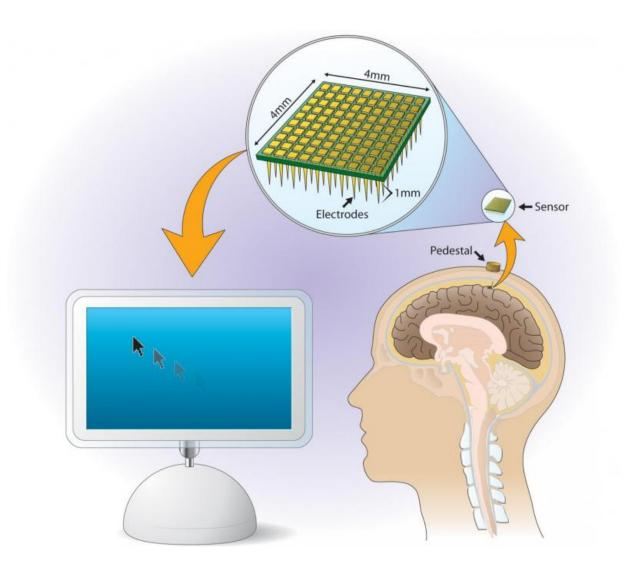
Neural signals recorded from an implanted array of electrodes are decoded to allow the participant to control a cursor on a computer screen by thinking about moving his own arm and hand. Credit: braingate.org
