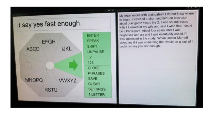
BrainGate2 clinical trial participant T6 used the brain-computer interface to control a specially designed radial keyboard. Innovations in the system's decoder keep the system calibrated automatically. Credit: Braingate.org
