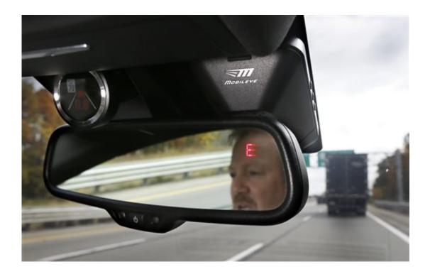
This Wednesday, Oct. 14, 2015 photo shows a Mobileye camera system that can be installed in your car to monitor speed limits and warn drivers of potential collisions, mounted behind the rearview mirror during a demonstration of the system, in Ann Arbor, Mich. (AP Photo/Carlos Osorio)
