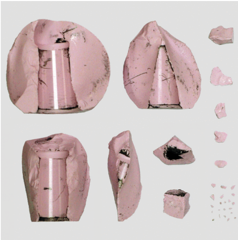
A picture of fragments of a fractured ceramic femoral head. Credit: JBJS Case Connector
