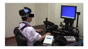
Set up for a brain computer interface rehabilitation system incorporating transcranial direct current stimulation. Credit: Elsevier
